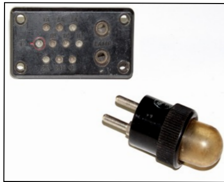
Valve test panel R107 showing position of lamp socket.
